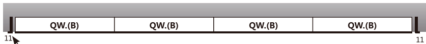
QW.(B) 段不含端盖，首尾端盖厚度各 11mm QW.(B) part without end cap, end cap width is 11mm at the beginning and the end
