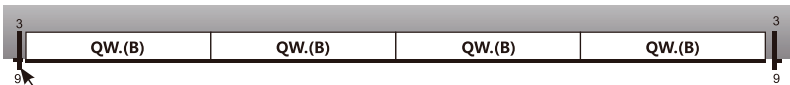
QW(B) 段不含端盖, 首尾端盖厚度各 9 mm QW(B) part without end cap, end cap width is 9 mm at the beginning and the end
