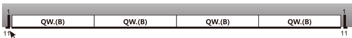
QW(B) 段不含端盖, 首尾端盖厚度各 11mm QW(B) part without end cap, end cap width is 11mm at the beginning and the end
