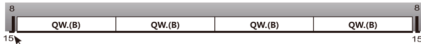
QW.(B) 段不含端盖, 首尾端盖厚度各 15mm QW.(B) part without end cap, end cap width is 15mm at the beginning and the end
